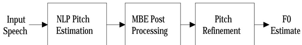
Figure 4.1: Pitch Estimation Block Diagram
